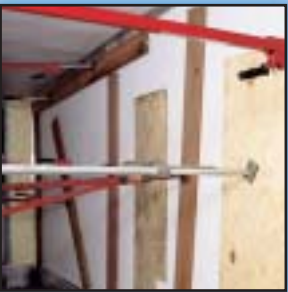
► Liner placed onto trailer wall. Bracing installed to maximize bonding process
