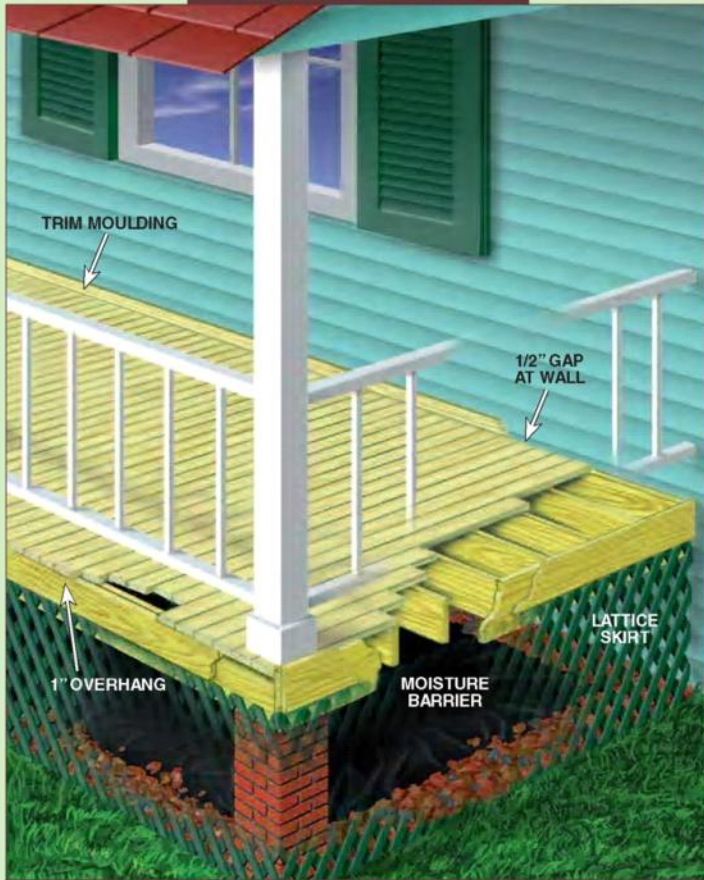
Figure 14: Porch Flooring Details
